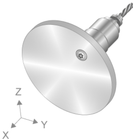
Fig. 115: Eccentric disc kinematic with rotation about X
