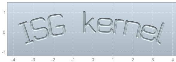
Fig. 96: Example of an arc layout, circle centre point is below the text
