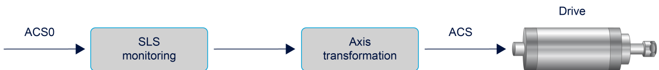
Fig. 54: Input of backward transformation with SLS monitoring
